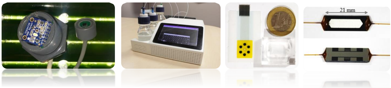
Fig. 2. Developed/adapted probes from left to right: RGB, turbidity, optofluidic system, electrochemical platform, preconcentrator chip for microGC.
