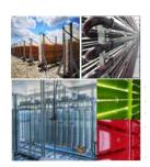
4 biorefinery scenarii - D. salina/6-carotene, T. lutea/fucoxanthin, H. pluvialis/astaxanthin, P. cruentum/zeaxanthin - were run at industrial scale, delivering altogether more than 200kgs of carotenoid-rich biomasses with high productivities up to 1g/L/day and high concentrations up to 10g/L. A proof-of-concept was also established for continuous production of light terpenes using GM-cyanobacteria.
